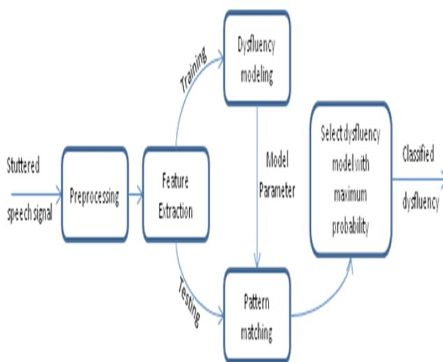
**Figure 2.** General block diagram of stuttering recognition system.
